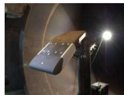
ASA WLE Demonstrator made of CMC coated with UHTC
