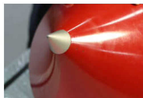
SHARK Structural aerodynamic profile made of massive UHTC
