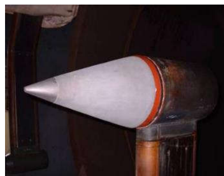
SHS Nose Cap Demonstrator: the tip is made of massive UHTC
